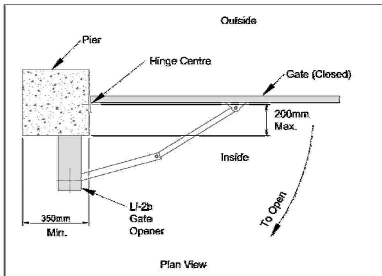
Figure 1: Standard installation.
