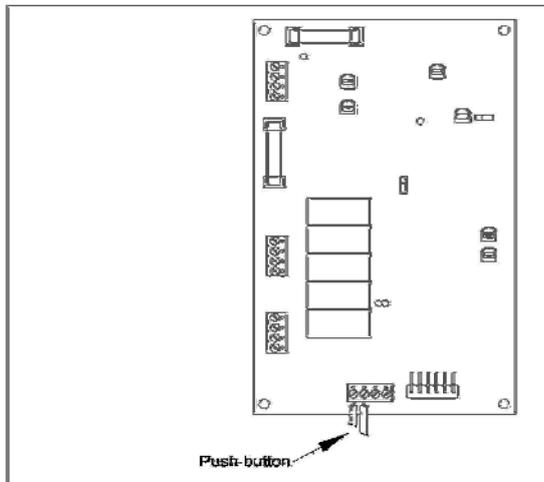
Figure 10: Push-button connection.
