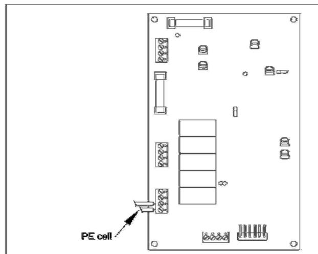
Figure 12: Photoelectric cell connection.
