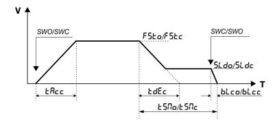
The V axis is the gate/door speed, T axis is the time required by the door/gate to move from a limit switch to the other (SWO to SWC and vice versa). The opening and closing phases have separate parameters, speed and decelerations can be adjusted differently. At gate/door stopped on any SWO (or SWC) limit switch, when a control key is pressed the gate/good starts moving and reaches the standard operating speed, which can be adjusted by FSTO/FSTC parameter.
