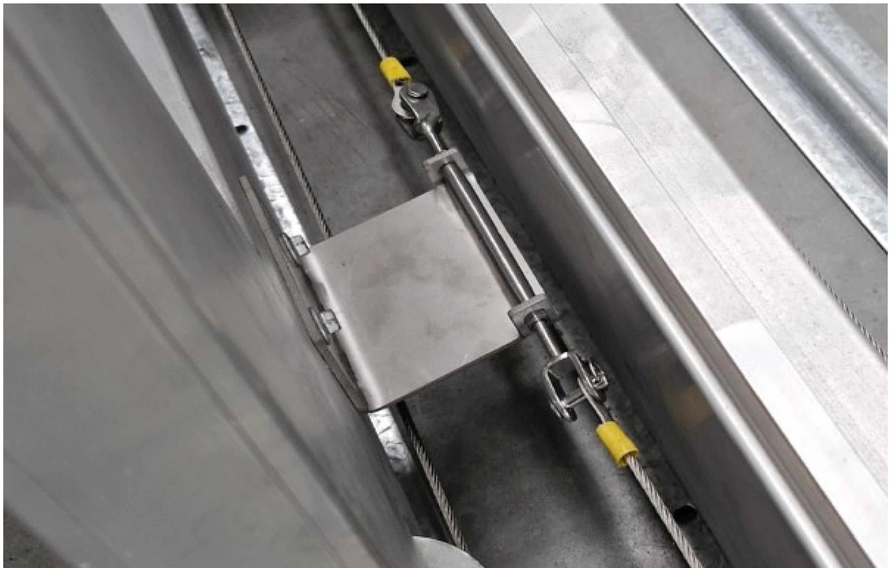
Cable clamp plate (2) - Fixes to gates two and gate three. Cable clamp bolts (4) - Two for each clamp plate.
