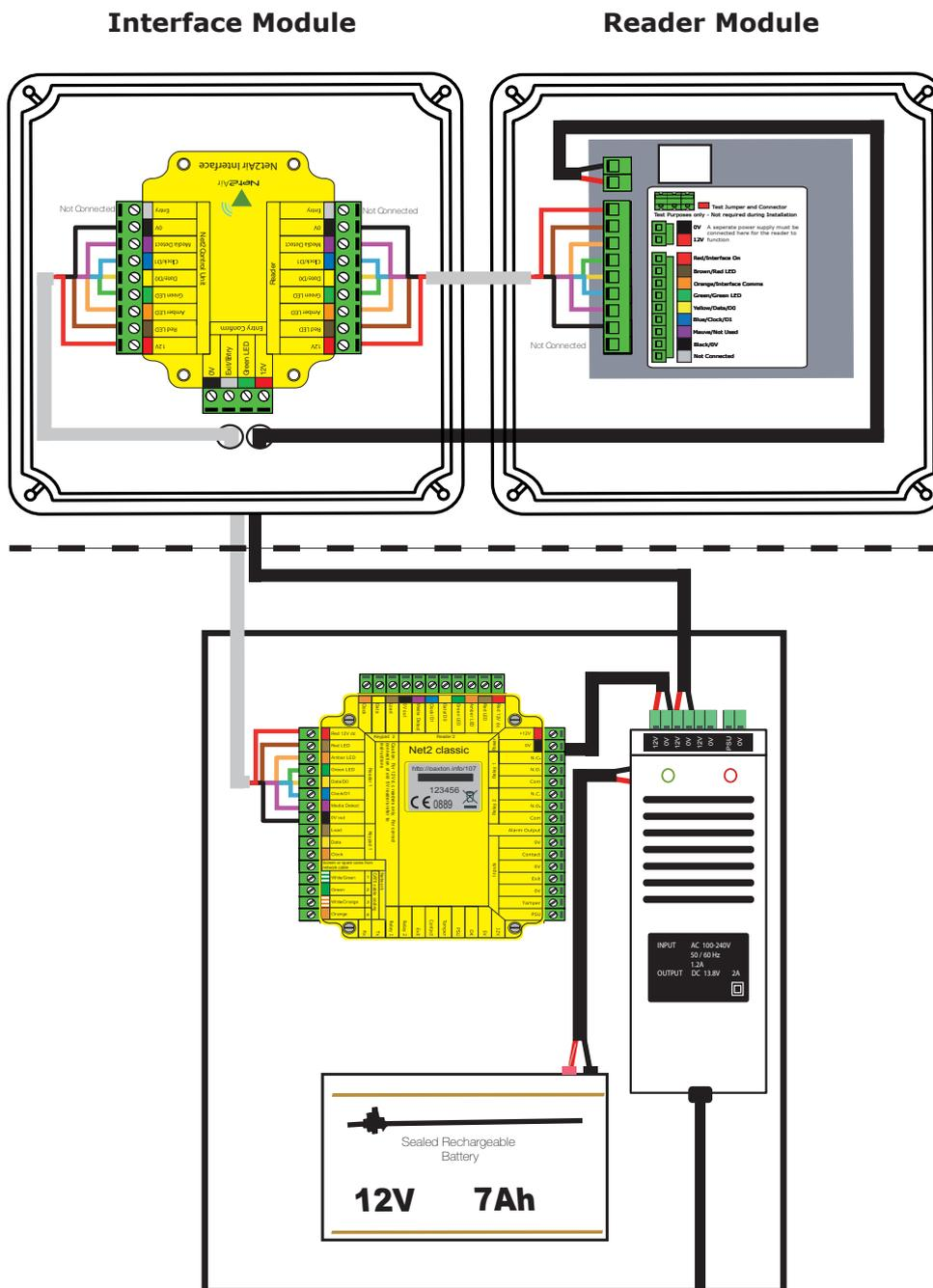
You will see that the interface is mounted upside down in the housing. This is to position the internal aerial away from other reader components and is intentional.
