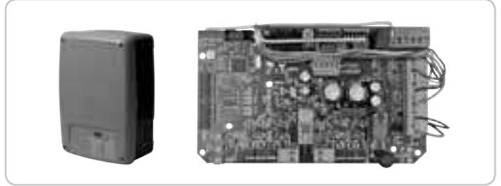
Control panel with impact sensors and MASTER Wi-Fi card.
