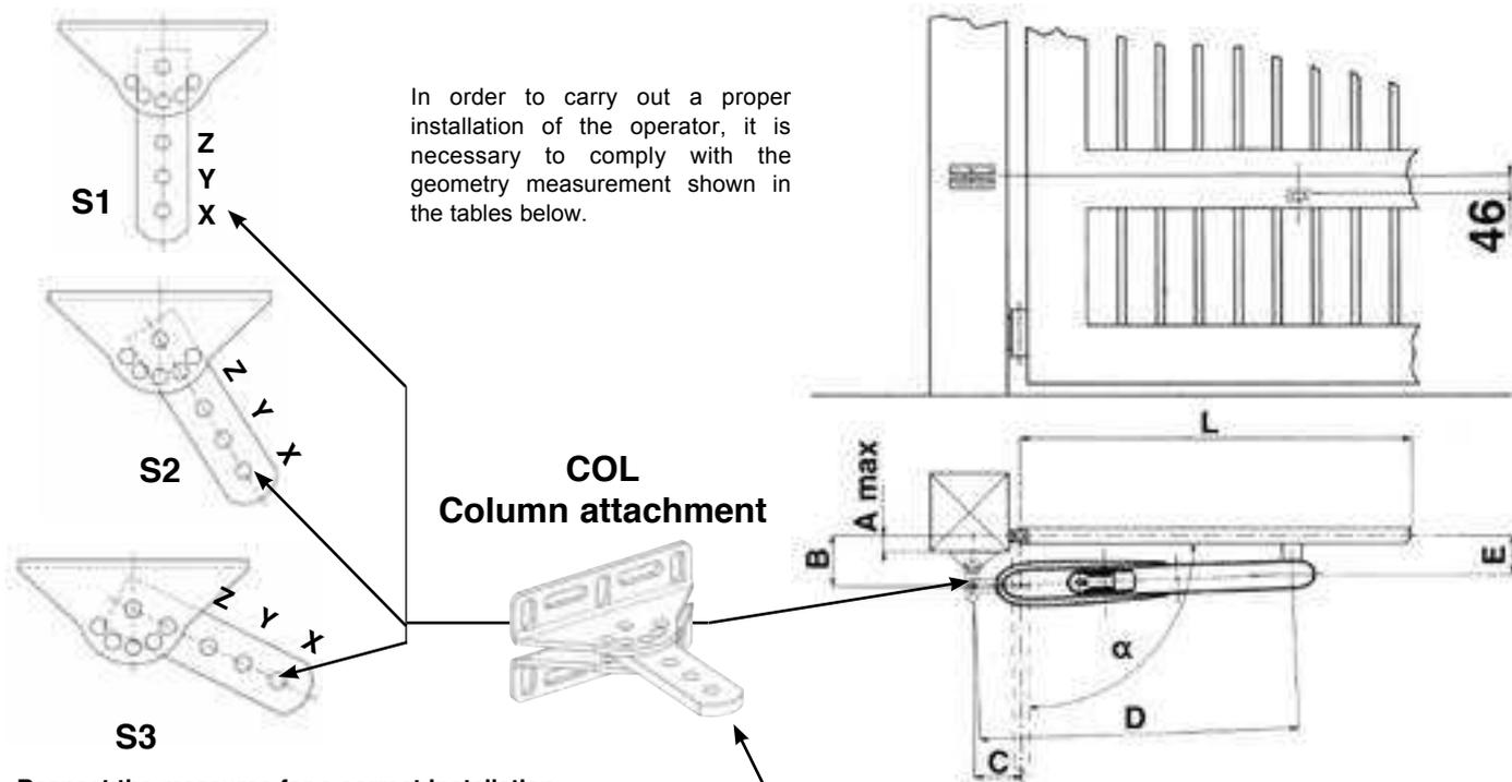
In order to carry out a proper installation of the operator, it is necessary to comply with the geometry measurement shown in the tables below.
