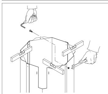
3 - Before fixing the upper flange, insert the metallic protection of the 50 mm diameter corrugated pipe which must be set in the ground to make the subsequent electrical connection with the control unit. See figures alongside.
