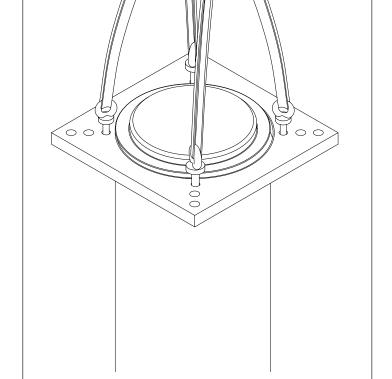
12 - Use four eyebolts with M8 studs to lift the bollard. See figures alongside.
