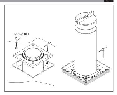
14 - Verify that the distance between the bollard flange and the upper edge of the case/flooring is equal to  $23\hbox{-}24~\text{mm}.$
