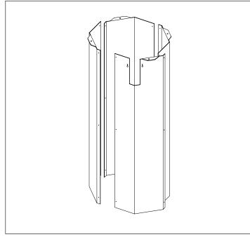
2 - Using the round head screws provided, assemble the hexagonal structure. It is very important to assemble the 4 elements vertically and on a surface that ensures excellent flatness so as to obtain a reliable support surface for the closing flange. Attention: The screw head must be placed on the internal side of the foundation case. See figure alongside.
