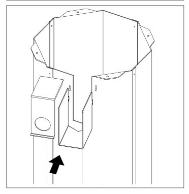
4 - Fix the upper flange using the round head screws provided. Attention: The screw heads must be placed on the upper part of the flange (inside the case).
