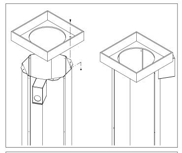
5 - Fit the clamps as in the figure locking them in position with the washer and the M10 hexagonal head screw. Fold them according to the foundation.
