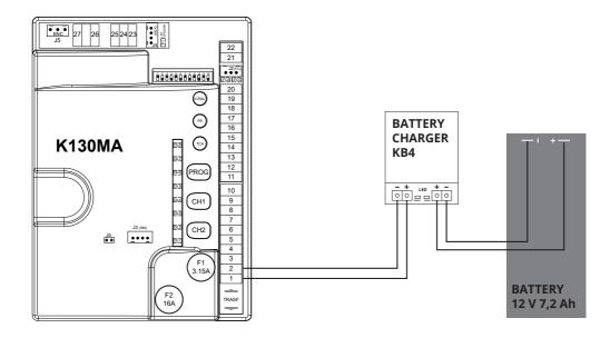
To ensure the gate operation during a power failure, the KB4 kit (battery charger + battery 12V 7.2Ah) can be used to connect to the control unit as shown in the diagram above.
