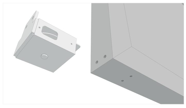
Fix or weld onto the two sides of the gate the boxes with the pulley.
