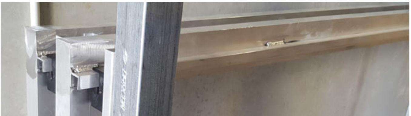
This completes fabrication of the main frame. The next step depends on gate design. In most cases you might complete the infill and/or pre drill and cut some of the installation holes before powder coating or painting.
